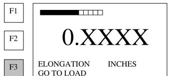
2. Press F3 (GO TO LOAD) to toggle to measurement of load.
