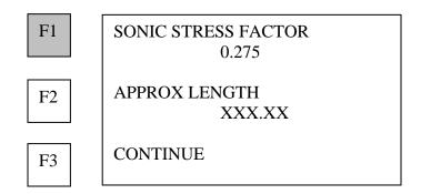
1. Press F1 (SONIC STRESS FACTOR) to change the sonic stress factor for the bolt type being measured.
