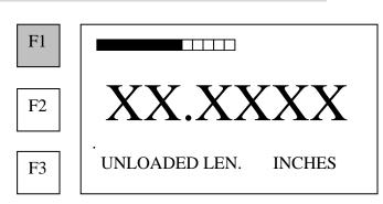
1. Press F1 for a graphic comparison of the present signal to the signal used for unloaded length measurement.
