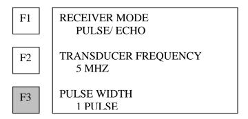
2. Press F3 (PULSE WIDTH) to scroll through the available settings for the width of the tone burst (number of pulse contained in each burst) transmitted to the transducer by the USM-3 tone burst pulser.
