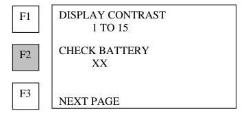
The percent of full charge remaining in the batteries appears below CHECK BATTERY.
