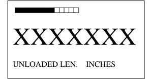
6. Press the ENTER key to place unloaded length measurement in memory. The USM-3 allows continuous measurement of a selected bolt, or sequential measurements of all bolts in the active Bolt Group.
