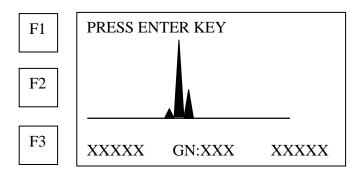
The operator should adjust the position of the transducer on the bolt end so the gain displayed in the lower portion of the display is the minimum achievable value, and the rectified display of the echo is, as close as possible, a single spike, of maximum height.
