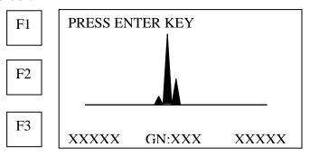
4. Adjust the position of the transducer on the bolt end to minimize the gain value displayed, and obtain, as closely as possible, a single spike of Maximum height.
