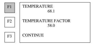
2. Press F1 (TEMPERATURE) if the temperature of the calibration bars at the time of use is different from the temperature shown.
