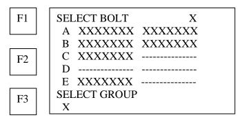
The USM-3 displays a tabulation of the 5 (A thru E) elongation and load readings recorded for the first bolt in the active Bolt Group. If no value is recorded for any of the measurements in the tabulation, the USM-3 will display dashes in the appropriate location.
