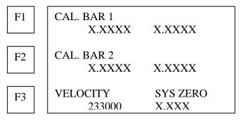
To verify that the system zero factor has been properly determined, check to see that the known length and ultrasonic length displayed, match to within  $\pm 0.0002$  inch or  $\pm 0.002$  mm. Repeat the ultrasonic measurements to verify.
