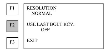
1. Press F2 (USE LAST BOLT RCV.) to toggle this function off and on.
