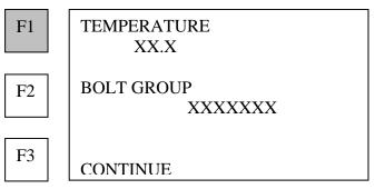
1. Press F1 (TEMPERATURE) to enter the bolt temperature
