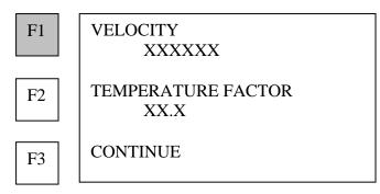
Note: The USM-3 defaults to the average velocity for steel: V= 232000 inches/sec (5892800 mm/sec).
