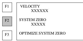
1. Press F2 (SYSTEM ZERO) to manually input a delay value for the system.
