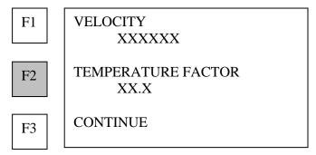
1. Press F2 (TEMPERATURE FACTOR) to change the value of the temperature factor.
