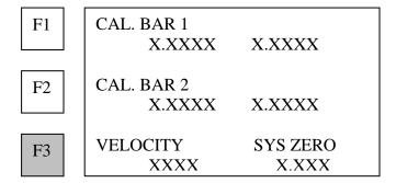
1. Press F3 (VELOCITY SYS ZERO). VELOCITY F1 XXXXXX **SYSTEM ZERO** F2 XXXXX **OPTIMIZE SYSTEM ZERO** F3 2. Press F1 (VELOCITY) to input material velocity other than that shown. **VELOCITY** F1 F2 XXXXXX F3 PRESS ENTER KEY 3. Enter data with number keys. 4. Press the ENTER key. VELOCITY F1 232000 **SYSTEM ZERO** F2 XXXXX **OPTIMIZE SYSTEM ZERO** F3 5. Press Back to return to calibration data menu F1 CAL. BAR 1 X.XXXX X.XXXX CAL. BAR 2 F2 X.XXXX X.XXXX VELOCITY **SYS ZERO** F3 XXXX X.XXX
